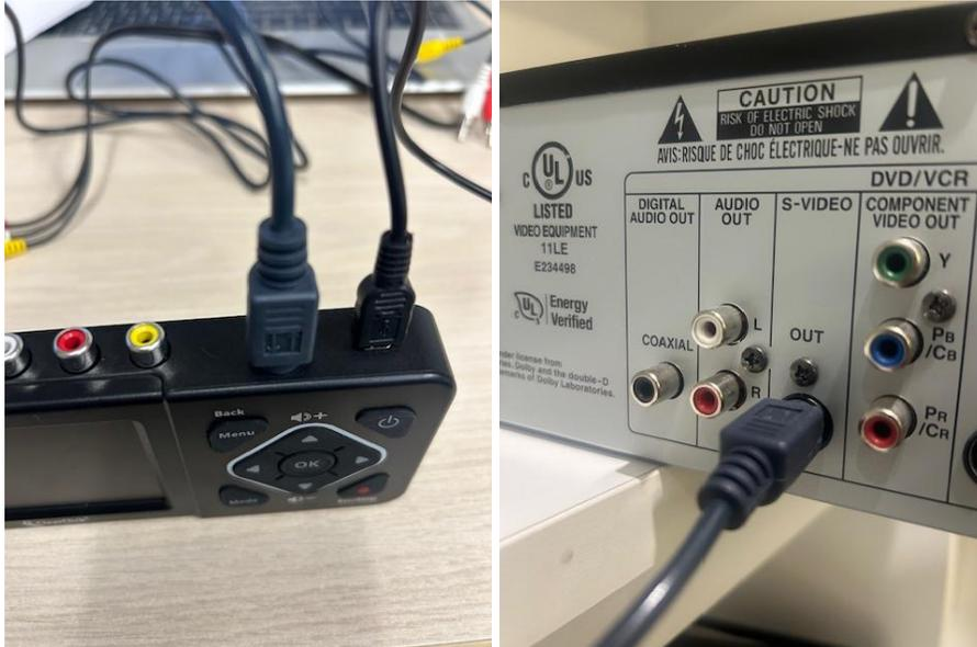
4. Attach audio source – Yellow, Red, White - to device and to the output option on the back of the VCR.
