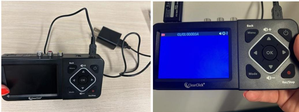
2. Plug in USB drive or SD drive. The USB plug in is on the top of the device, the SD is on the side.
