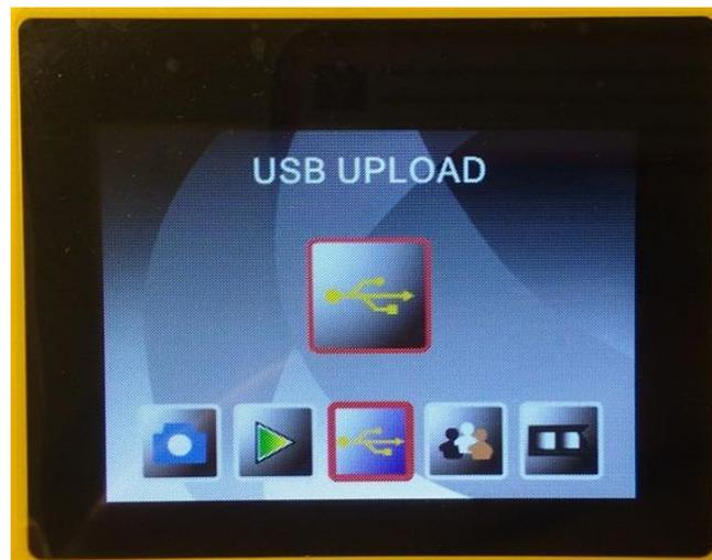
Press **OK/Enter** and the converter will connect with the computer. You can now save your slides on a USB stick.
