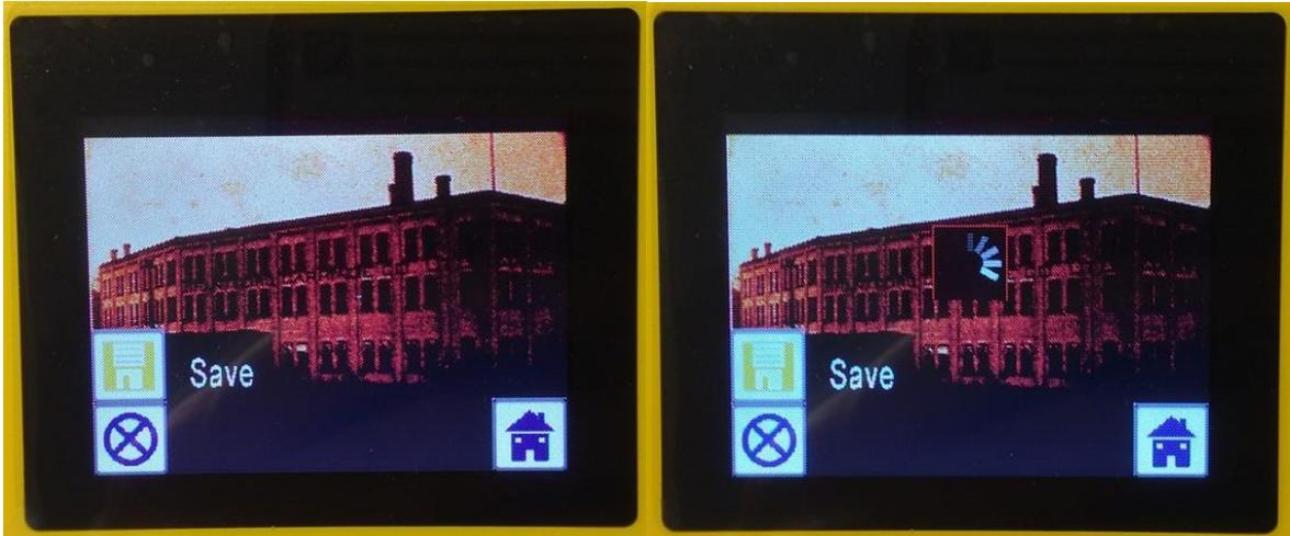
To convert and save your slide press **Convert/Mode**. **Save** will be highlighted and press **OK/Enter**. It will take a few seconds for your slide to be converted and saved.
