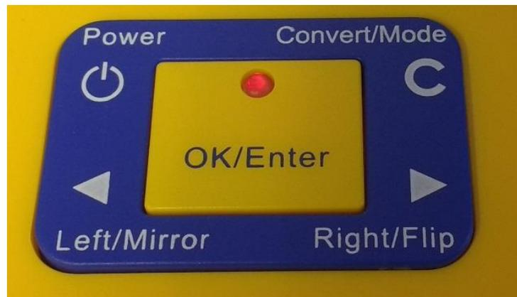
**Film Type** will be displayed on the screen. Press **OK/Enter** and **Slide Positive** will be displayed on screen. Press **OK/Enter** again to select **135** (35 mm - the most common for regular slides)
